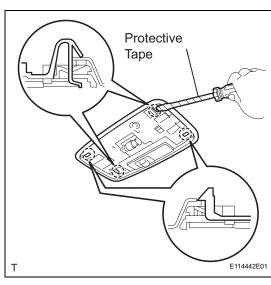
(c) Using a screwdriver with its tip wrapped in protective tape, disengage the 4 claws.
